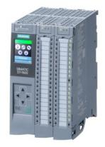
\*\*\* Spare part \*\*\* SIMATIC S7-1500 Compact CPU CPU 1511C-1 PN, central processing unit with work memory 175 KB for program and 1 MB for data, 16 digital inputs, 16 digital outputs, 5 analog inputs, 2 analog outputs, 6 high-speed counters, 4 high-speed counters for PTO/PWM/frequency output 1st interface: PROFINET IRT with 2-port switch, 60 ns bit performance, incl. push-in front connector, SIMATIC Memory Card required
