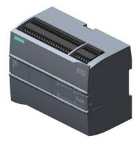
SIMATIC S7-1200, CPU 1215C, compact CPU, AC/DC/relay, 2 PROFINET ports, onboard I/O: 14 DI 24 V DC; 10 DO relay 2 A, 2 AI 0-10 V DC, 2 AO 0-20 mA DC, power supply: AC 85-264 V AC at 47-63 Hz, program/data memory 200 KB
