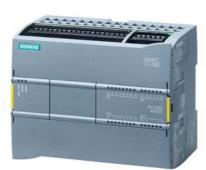
SIMATIC S7-1200F, CPU 1215 FC, compact CPU, DC/DC/DC, 2 PROFINET ports, onboard I/O: 14 DI 24 V DC; 10 DO 24 V DC; 0.5 A; 2 AI 0-10 V DC, 2 AO 0-20 mA DC, power supply: DC 20.4-28.8 V DC, program/data memory 250 KB
