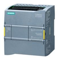
SIMATIC S7-1200F, CPU 1212 FC, compact CPU, DC/DC/DC, onboard I/O: 8 DI 24 V DC; 6 DO 24 V DC; 2 AI 0-10 V DC, power supply: DC 20.4-28.8 V DC, program/data memory 150 KB
