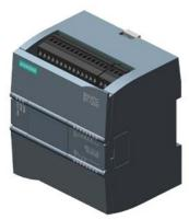
SIMATIC S7-1200, CPU 1211C, compact CPU, DC/DC, onboard I/O: 6 DI 24 V DC; 4 DO 24 V DC; 2 AI 0-10 V DC, Power supply: DC 20.4-28.8V DC, Program/data memory 30 KB
